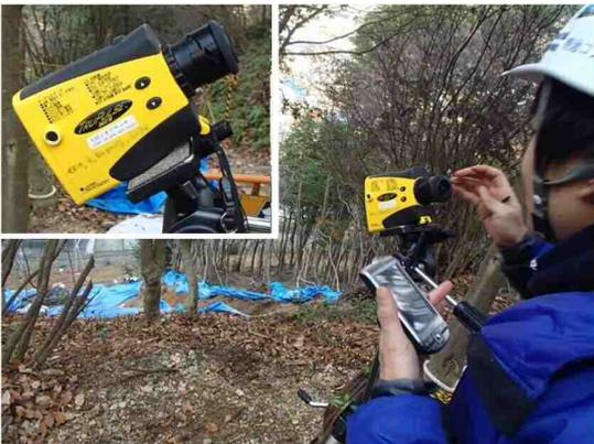
Fig.7 Topographical survey using reflectorless laser measurement tool
