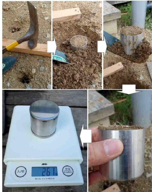
Fig.4 Unit weight test using circular cylinder
