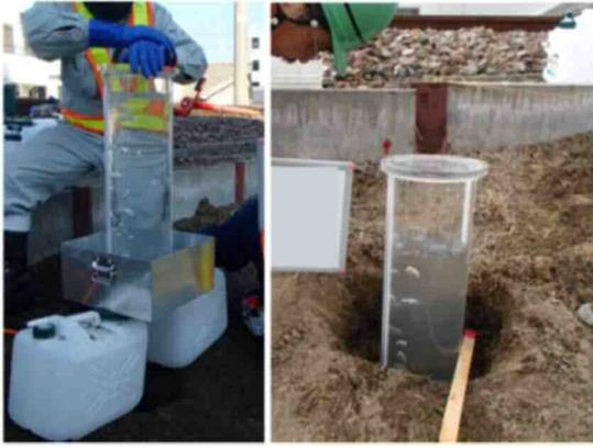
Fig.5 On-site permeability test
