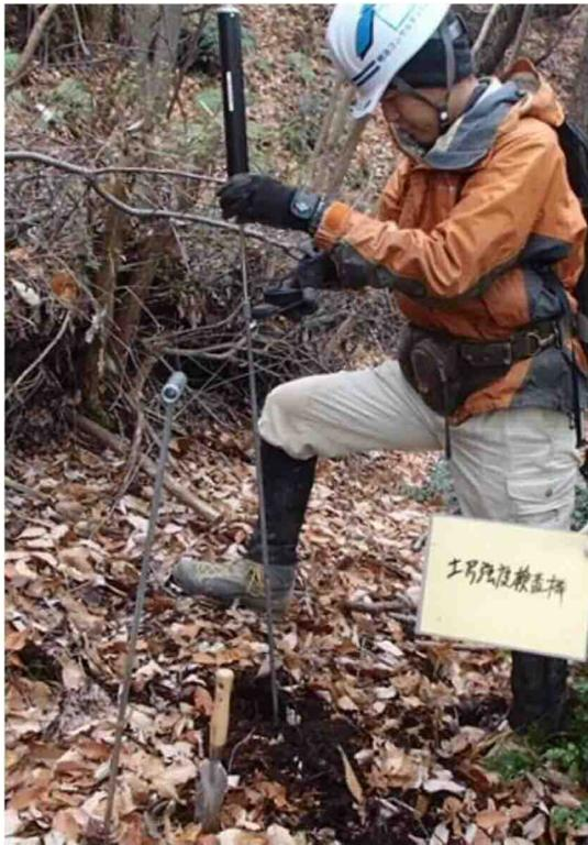
Fig.1 On -site Soil Strength Probe Test (SSPT)
